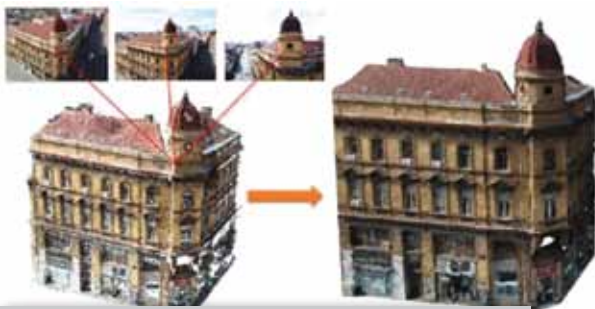
Example of the use of photogrammetry in building analysis
