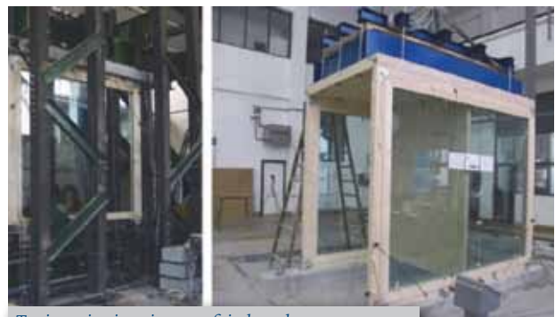
Testing seismic resistance of timber-glass systems
