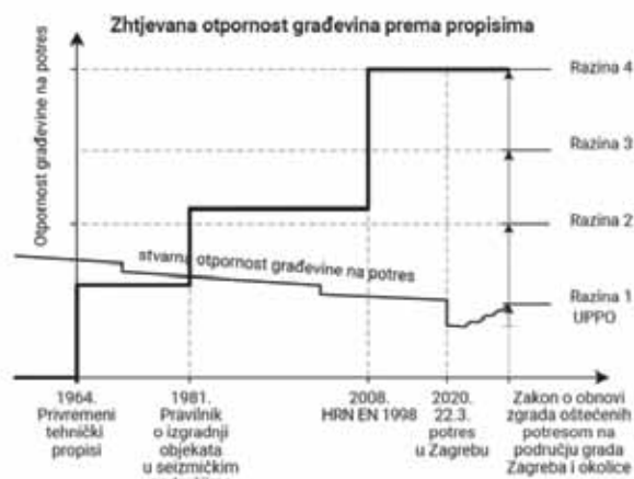
Schematic view of reconstruction levels as related to bearing capacity of buildings (adopted from UERP)
